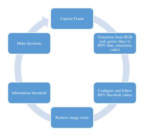
Figure 1 Diagram demonstrating the process for detecting a reference object
